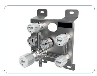
The Spec Master HPM6010 Series single stage single cylinder manual change control panels are designed for primary pressure gas control of non-corrosive or toxic, high purity gases up to grade 6.0 purity (99.9999%), on gas distribution systems where slight pressure variation is acceptable.
